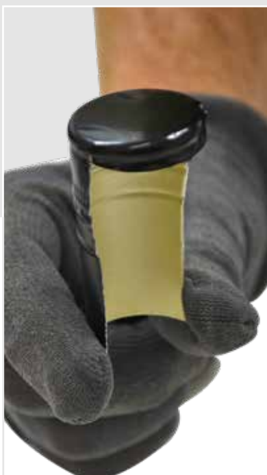
6 - Preparation of the cut cap for calibration of the rolling head rollers.
